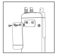
**CAUTION:** Do not tighten the screws too tight. You could damage the case or clip.
